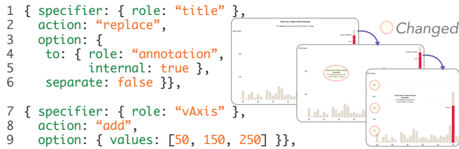
Figure 10: An example use case (Disaster Cost) for our Cicero compiler's default behavior for replacing the title as an internal annotation (line 1–6) and for introducing newly added elements (axis labels and grid lines; line 7–9).
